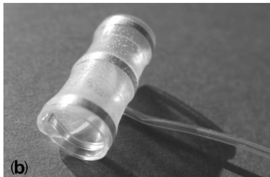
Figure 3.1: Schematic representation of electrode placement (a) and the electrode cuff (b). In all fifteen pigs, three cuffs were placed on the left vagus nerve. In four out of fifteen pigs, an additional recording cuff was placed on the right vagus nerve.
